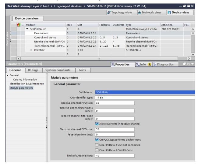
CAN bit rate: 10, 50, 100, 125, 250, 500, 800 Kbps, and 1 Mbps are available as bit rates.
