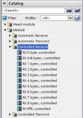
If changed data is not fetched from the PLC fast enough, the parameter "CAN-RX overwrite allowed" allows newly received telegrams to overwrite the data of the previous telegram that has not yet been fetched. The PLC then always receives the last data. If the parameter is not activated, new data are only taken over from the CAN bus when the PLC has fetched the data.
