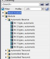
A CAN message always has a fixed data length. In the case of automatic reception, CAN messages with 1 to 8 bytes can be configured.
