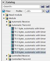
The repetition time enables a cyclic transmission of the CAN message with the actual data bytes.
