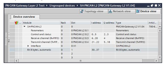
If a CAN message is received that has the correct CAN identifier but a false data length, the message is rejected, and the data is not forwarded to the PLC!
