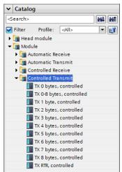
The module "TX 0-8 Bytes, controlled" can be used for sending CAN messages with different data lengths. In addition to the data, the length of the CAN messages can also be transferred to this module.
