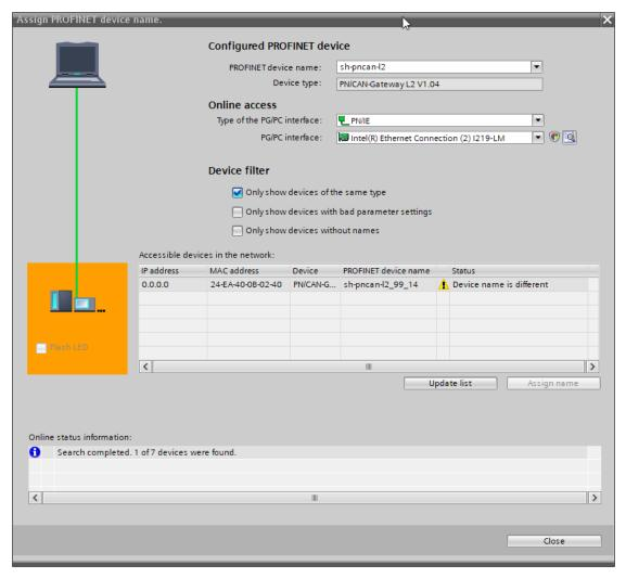
The clear identification of the PN/CAN gateway is ensured here by the MAC address of the device. The MAC address of the device is on the front of the PN/CAN gateway.
