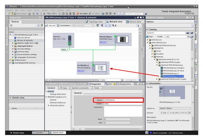
By calling up the object properties, the PN/CAN gateway should be assigned a unique PROFINET name and the IP address be checked for plausibility.
