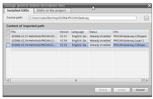
The PN/CAN Gateway can be found in the hardware catalog under "Other field devices → PROFINET IO → Gateway → Helmholz PN/CAN Gateways".
