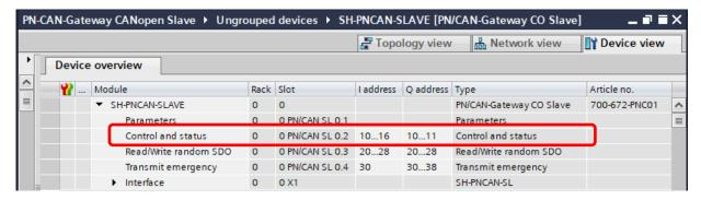
The most important function of the control and status bits is to control the CANopen slave state.
