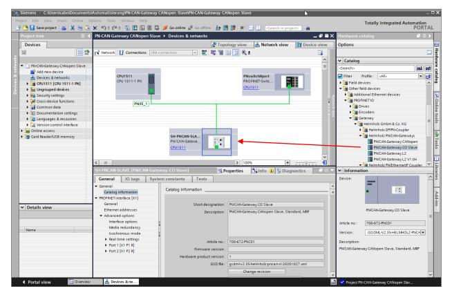
By calling the properties, a unique PROFINET name should be assigned to the PN/CAN Gateway and the IP address checked for plausibility.
