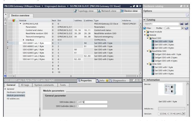
For the EDS example "DS401\_IO\_Slave\_Vxx.eds" the input SDO 6000 must be described from the PLC since these are readable values from the point of view of the CANopen network (inputs). The SDO 6200 can be read by the PLC since these are writable values from the point of view of the CANopen network (outputs).
