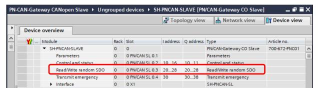
With this module an SDO can be accessed randomly on a command based exchanged.
