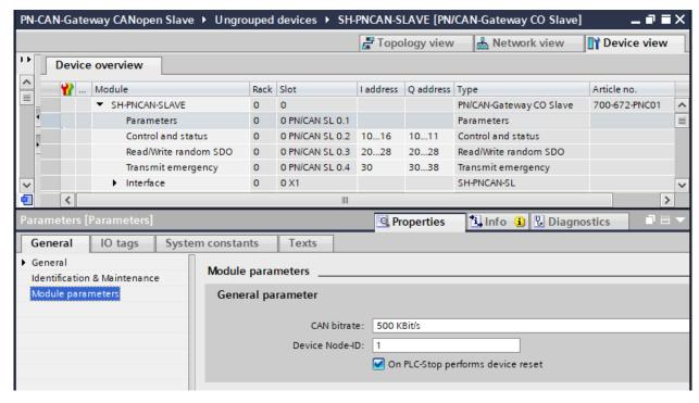
**CAN bitrate:** The available bit rates are 10, 50, 100, 125, 250, 500, 800 KBit/s and 1 MBit/s. When using a DCF file, this parameter is ignored, because the bitrate is supplied in the DCF file.
