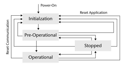
With the NMT command "Operational" [COB-ID:  $000_{\rm hex}$  / data (2 bytes):  $01_{\rm hex}$  node ID], a CANopen device can be switched to the operational status. Once in the Operational state, the coupler's process data will be enabled (RPDO/TPDO communications will be running). The options available for making changes to SDOs may be limited.
