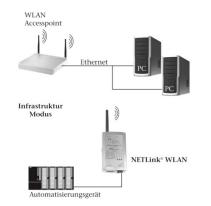
When using the infrastructure mode the communication of two WLAN components is handled by a mediation unit, an access point (AP). The AP functions as central coordination point of the
