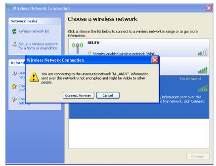
5. Step: The connection to NETLink<sup>®</sup> WLAN is now successfully established, and it can be implemented e.g. via the PG/PC interface parameterization.
