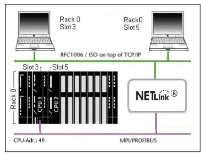
The rack/slot address for the station that will be used to communicate on the rack must be configured in the communication software (in the above example: R/S = 0/3 for CPU 1 and R/S = 0/5for CPU 2)
