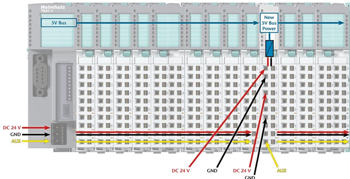
The order no. for the power module is 600-700-0AA01. The electronic module of the power module is light gray like the front connector. The base module of the power module is light gray with a dark top part.
