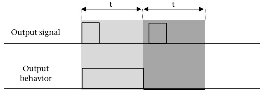
Example 2: Output signal is a series of short pulses.
