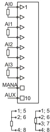
Mana = Masse ANAlog = analog ground = reference ground of the analog measurement
