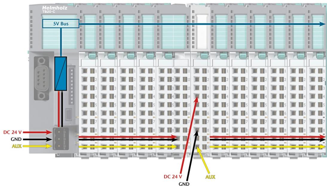
The order no. for the power and isolation module for 24 V signals is 600-710-0AA01.
