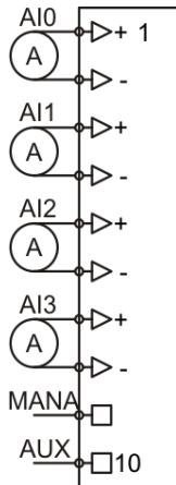
Mana = Masse ANAlog = analog ground = reference ground of the analog measurement
