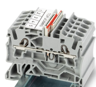
Orient the staggered jumpers' red stripes on the inside. Insert the staggered jumper and push down until it hits the backstop.
