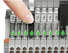
Configuration via push/slide switch
