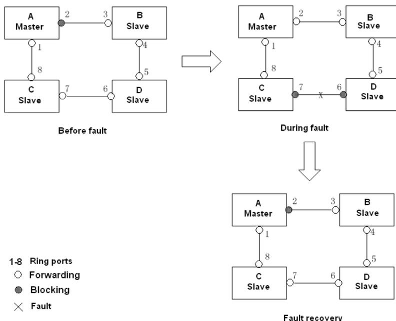
Figure 207 CD Link Fault
