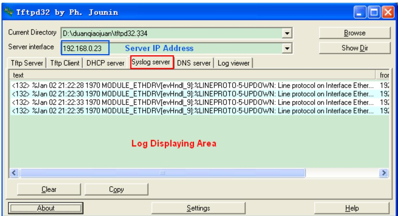
Figure 258 Uploading Log Information in Real Time
