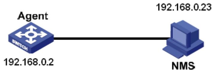
Figure 114 SNMP v2c Configuration Example
