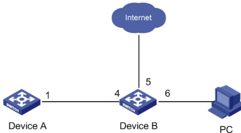
Figure 206 GVRP Configuration Example
