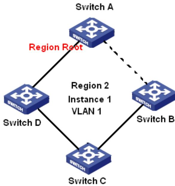
Figure 233 VLAN 1 Mapping to Instance 1
