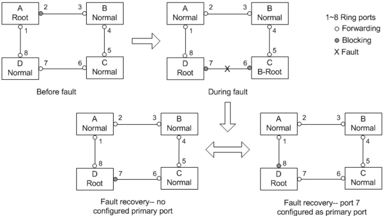
Figure 216 DRP-IEC62439 Link Fault
