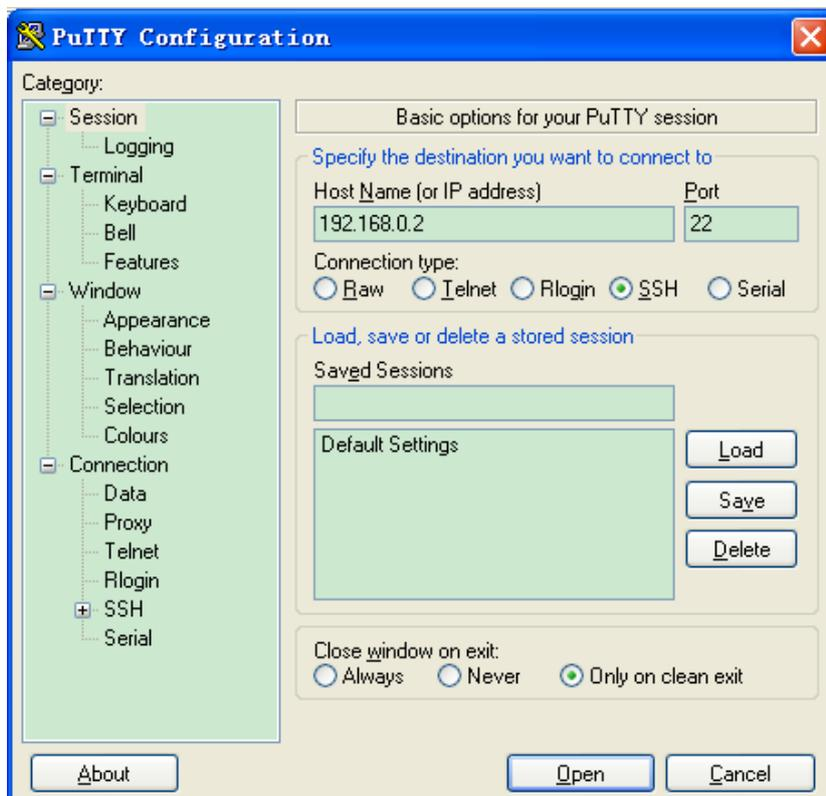
Figure 99 SSH Client Configuration
