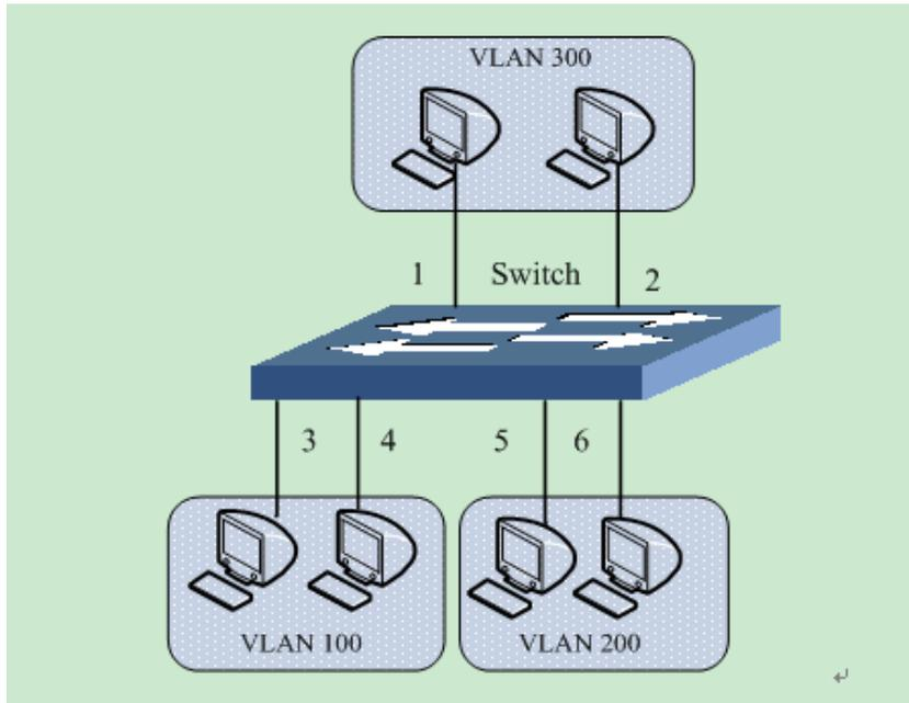
Figure 201 P VLAN Configuration Example
