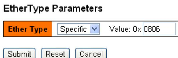
Figure 76 Configure the EtherType Frame Parameters
