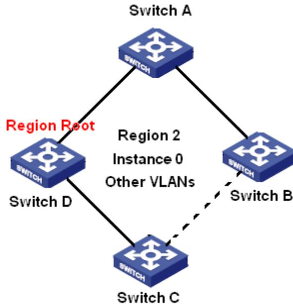
Figure 235 Other VLAN Mapping to Instance 0
