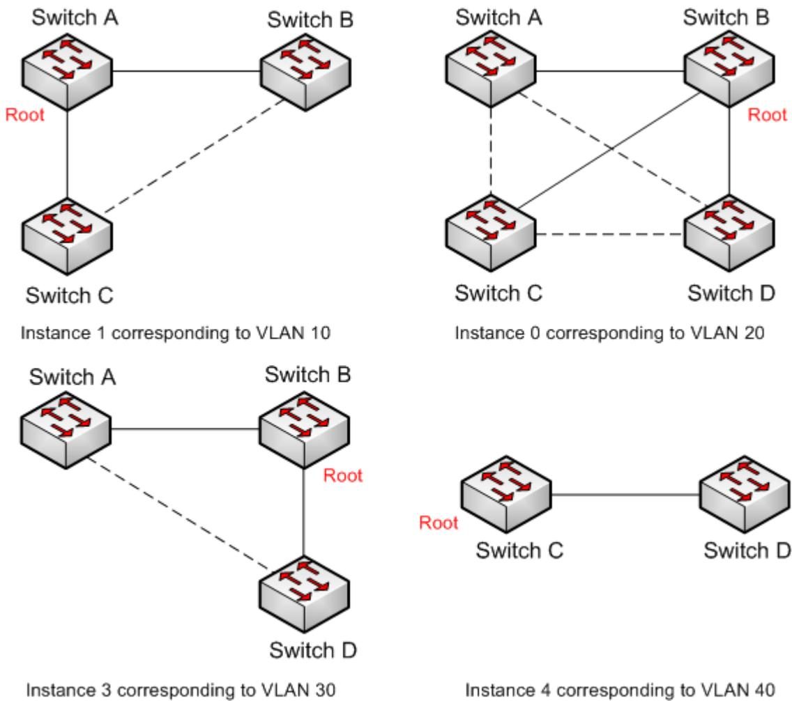
.....Blocked link through MSTP calculation
