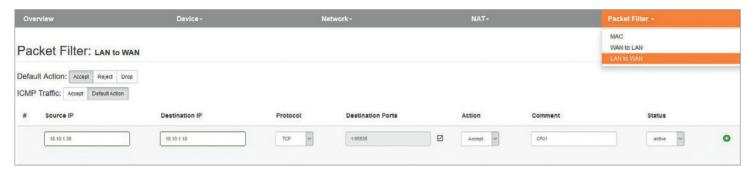
In the "LAN to WAN" packet filter, the communication of devices in LAN with devices in the production network (WAN) can be completely prohibited or be blocked or allowed for particular devices.
