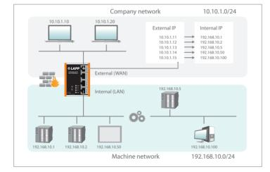
**Example:** A PC in the production network (WAN) has the IP address 10.10.1.11 (e.g. a visualization). This PC should be able to access the CPU with the IP address 192.168.10.1 within the LAN via the port 102 with the help of the TCP protocol.
