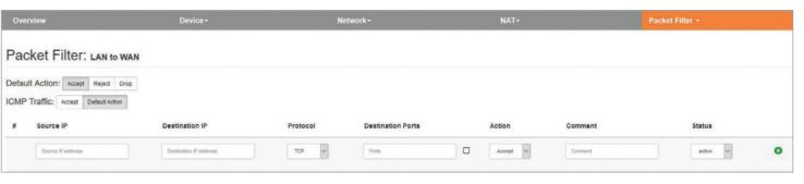
In the "LAN to WAN" packet filter, the communication of devices in LAN with devices in the production network (WAN) or into the Internet is completely prohibited or is blocked or allowed for particular devices.
