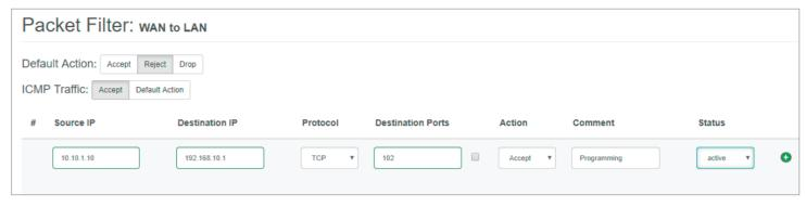
Source IP indicates the IP address of the active device in the production network (WAN). Destination IP the addressed device in the machine network (LAN).
