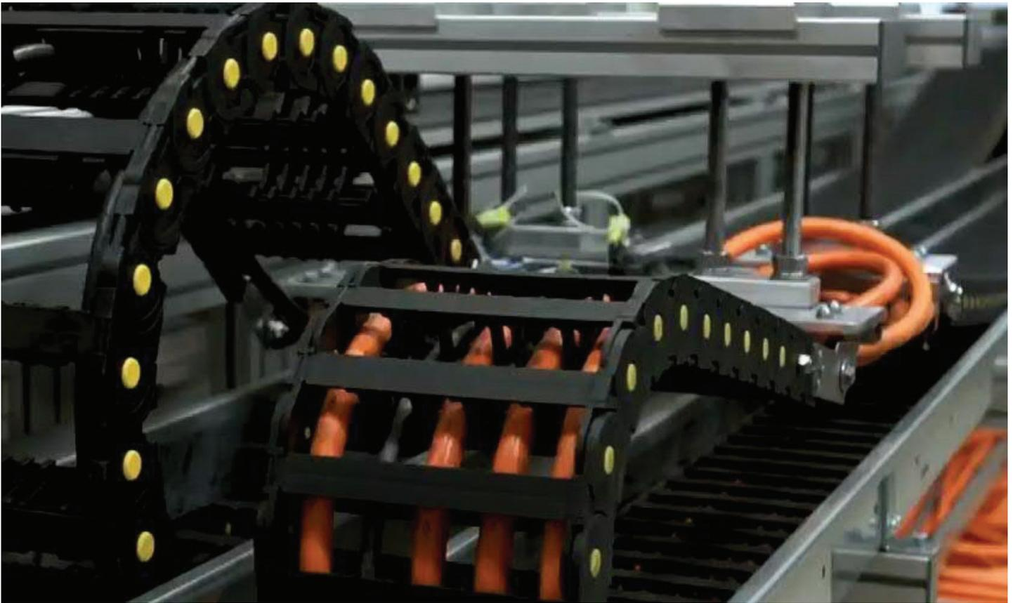
Cable tray requires cable tested for continuous flex. ÖLFLEX SERVO FD 7TCE is rated for continuous flex and can be installed in cable trays.
